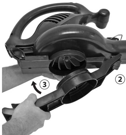
Figure 3-3: Attaching bottom inlet cover to motor housing hook
